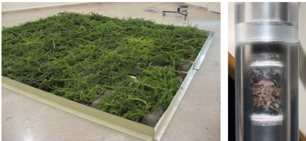
574 575 Fig. 13. Measurements of the sound absorption coefficient in the diffuse sound field (reverberation room) 576 and in the standing wave sound field (Kundt tube).
