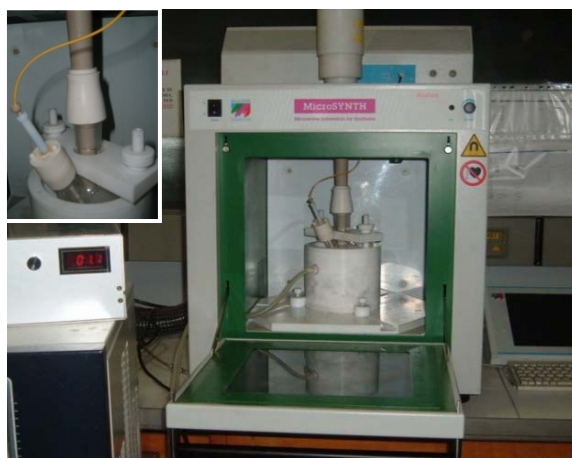
Figure 4. SMUI with a cooling system (Authors' lab)
