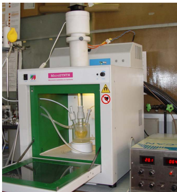
Figure 10. Transesterification under SMUI (Authors' laboratory).
