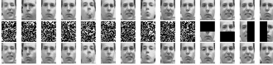
Figure 5: The first row shows the original images, second row shows the images with pixels missing, and the third row shows the reconstructed images.
