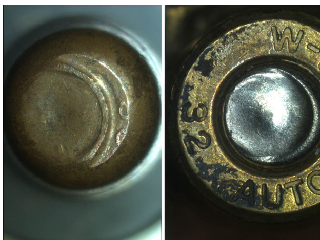
Fig. 5 Comparison between the “nose” of the 7.65 mm projectile found at the scene (to the left ) and the base of the 7.65 mm shell casing recovered from the body (to the right ); note the corresponding imprints
