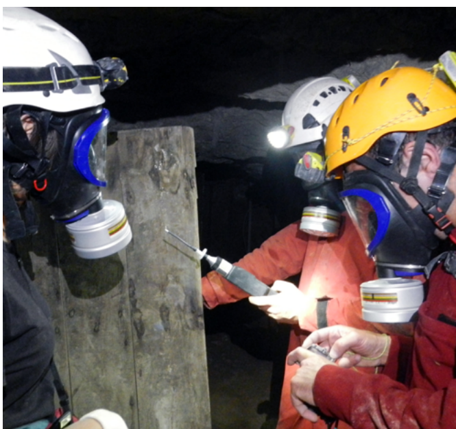
Fig. 14: check of level of dangerous gas before the access in the 5th level gallery (photo M. Vattano).
