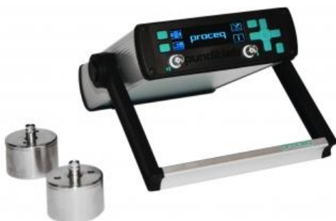
Fig. 4 – Particular of the sonotrode (a), built at this purpose by Sirius electric, and of the generator/receiver (Pundit lab by Proceq from Pasi srl).
