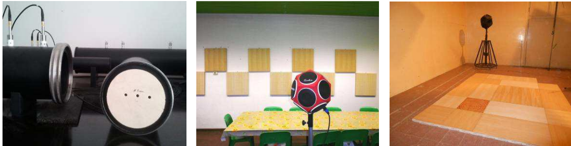
Figure 3: Main phases of the acoustic testing: on small specimens through impedance tube (left), on end-size samples in a dining room (center) and in reverberation room (right)
