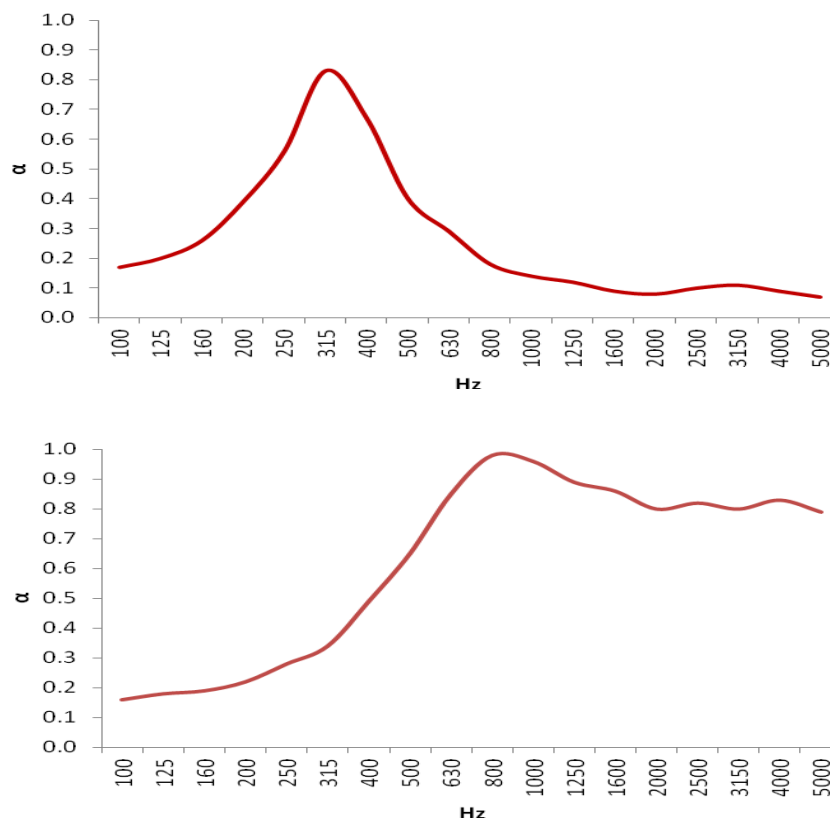
Figure 4: Examples of the sound absorption properties achieved by the acoustic panels (top) and by the bass traps (bottom)
