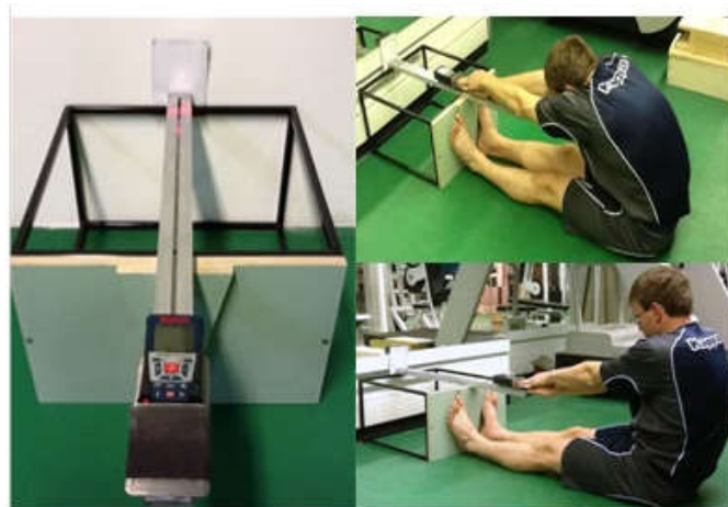
Figure 1. The new version of Sit and Reach Parallelepipedon with digital distance meter
