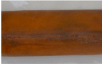
Rubber after the treatment with EVA4260
