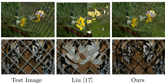
Fig. 12: Examples where Liu de-fencing approach [17] fails in fence detection or in removal phase 2 . Left: test image; Middle: fence detection results of Liu Algorithm; Right: de-fenced image using proposed approach.
