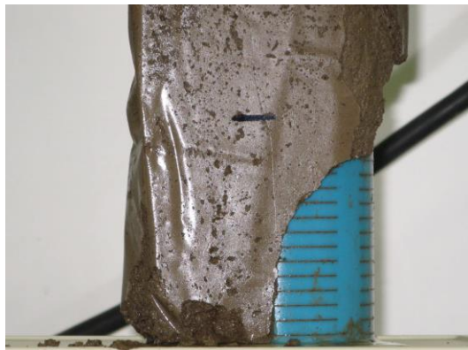
Fig 6 – Example of occlusion of the openings (slotting) on filter D1 with a mixture of earth and concrete.
