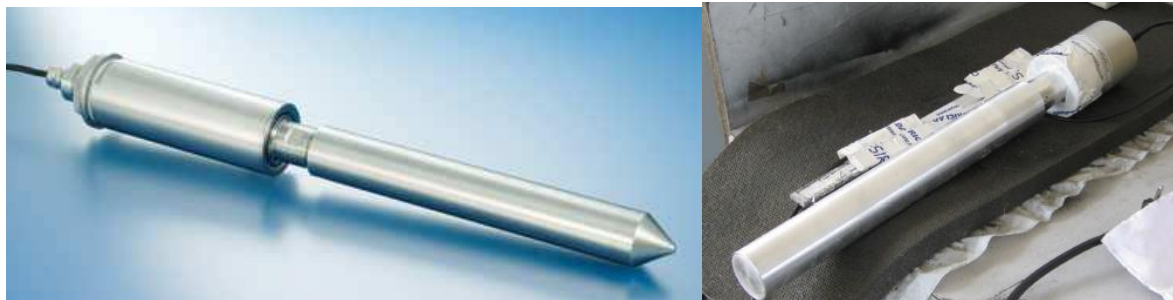
Fig. 5 - Weber Ultrasonic (sx) Sirius Electric (dx) sonotrodes used in lab tests.
