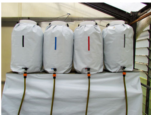
Fig. 4. Reservoirs for the new hydroponic nutrient solution (HNS) stocks.
