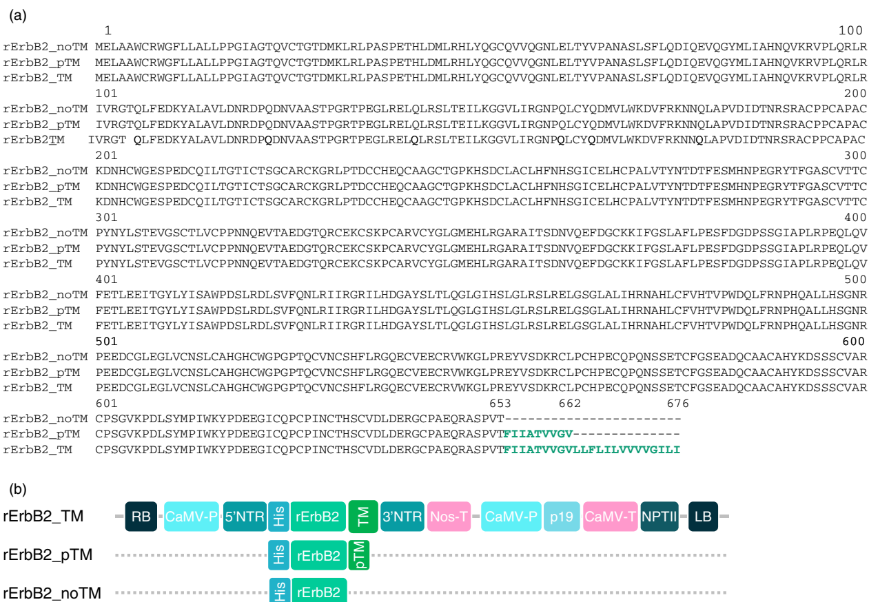
Figure 1 rErbB2 variants and constructs description. (a) ClustalW alignment of the EC domains of the rErbB2 proteins, with the TM domain indicated in green. (b) Scheme of the T-DNA regions within the right and left borders (RB and LB). The rErbB2 synthetic genes fused to the 6X His tag (His) of pEAQ-HT are under the control of the CaMV promoter (CaMV-P), between the 5' and 3' untranslated regions (NTR) of the RNA-2 of Cowpea mosaic virus and the nosipalme synthase terminator (Nos-T). pEAQ-HT also includes the silencing suppressor p19, under CaMV promoter and terminator (CaMV-P and -T).
