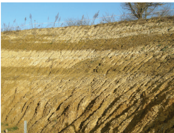
Fig. 13 - Clayey silt with a hint of planar bedding, evidenced by different carbonate contents: the light horizons show a cementation and are rich of pedogenetic carbonatic concretions; the dark horizons (brown color 7,5 YR 5/8) appear strongly cemented by iron oxides and rich of pseudogleys. Outcrop of Maretto Unit N of Palazzo Gianotti (central sector of the type-
