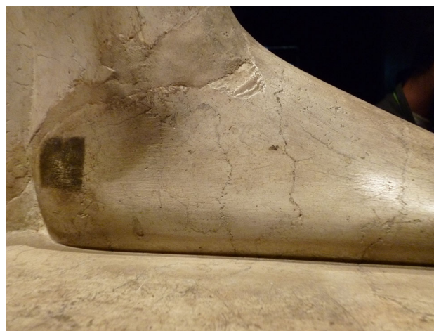
Fig. 7 Detail of the statue of Amon (Cat. 0768) made of fine-grained limestone. Stylolites are clearly recognizable as indented dark surfaces
