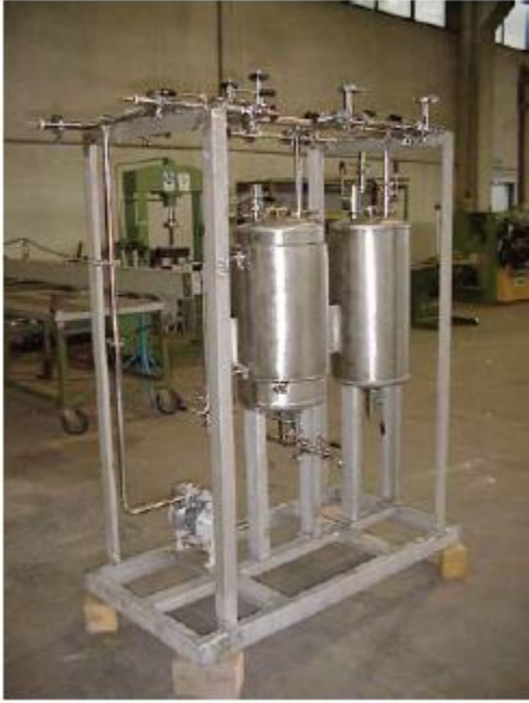
Figure 1. Hydrodynamic cavitation pilot unit
