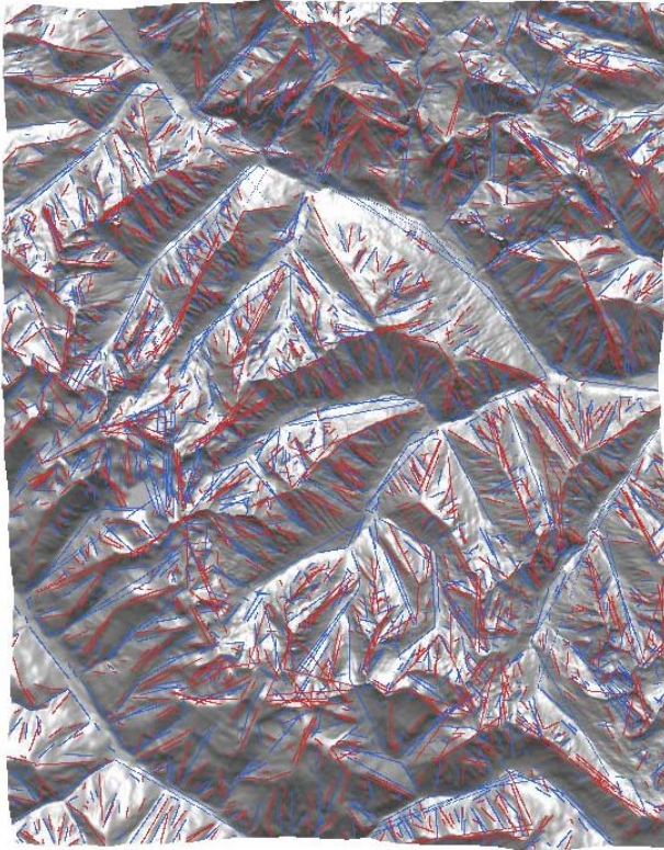
Figure 3. Image of Bagni di Vinadio DTM with all lineaments extracted by CurvaTool
