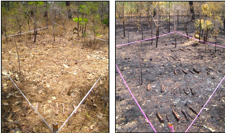
Figure 5-12 Replicates and log sets before (left) and after (right) burning
