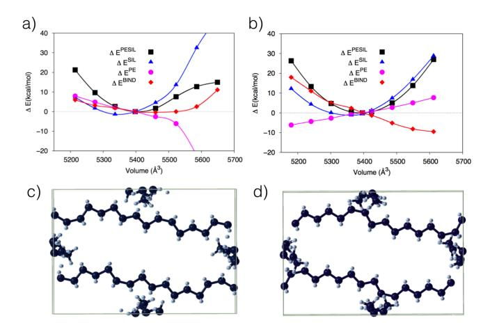
**Figure 2** Energy decomposition of contributions to the total energy of PESIL before (panel a) and after (panel b) relaxation of strains in the polymeric (PE) moiety, reported as a function of the unit cell volume. In panels c) and d) changes in the conformation of the polymeric chain, before and after relaxation respectively, are clearly visible.
