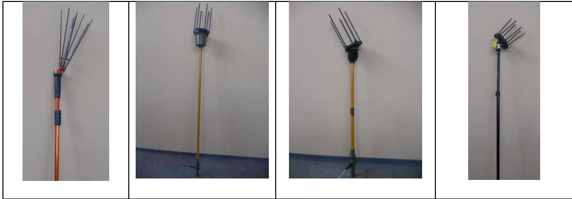
Figure 2. The hand held olive harvesters studied in this work (from left to right: C2, B1, B2, A1). The C1 beater is omitted because it has the same shape of C2.
