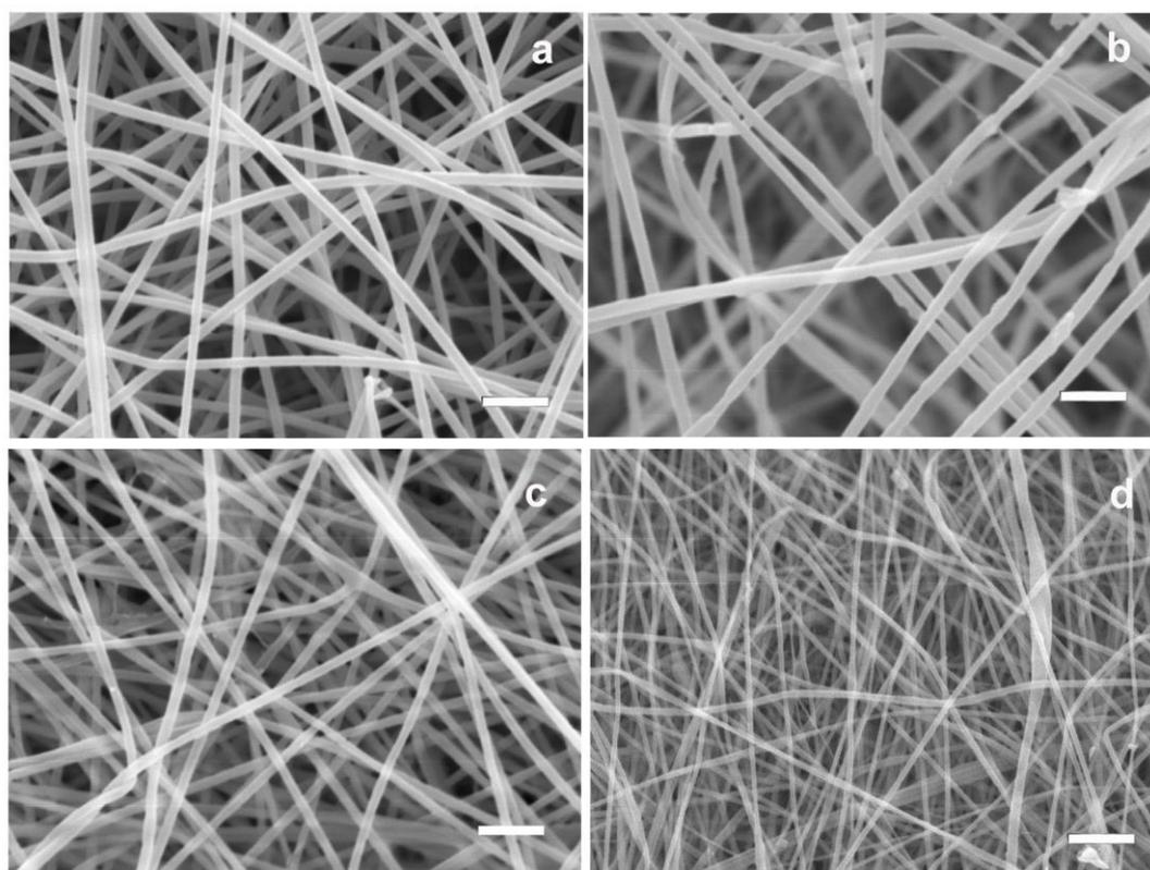
**Figure 7.** Scanning electron microscopy of electrospun gelatin-GO mats a) M-0, b) M-0.5, c) M-1. d) M-1.5. Scale bar: 5  $\mu\text{m}$ .
