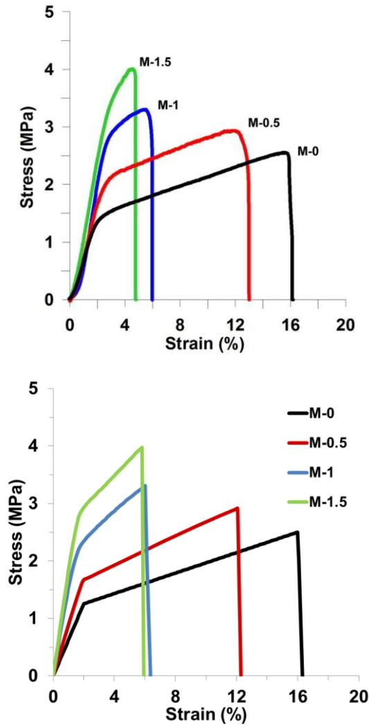
**Figure 9.** a) Representative stress strain curves of gelatin-GO nanofiber mats as a function of the composition. b) Corresponding numerically calculated Stress-Strain curves.
