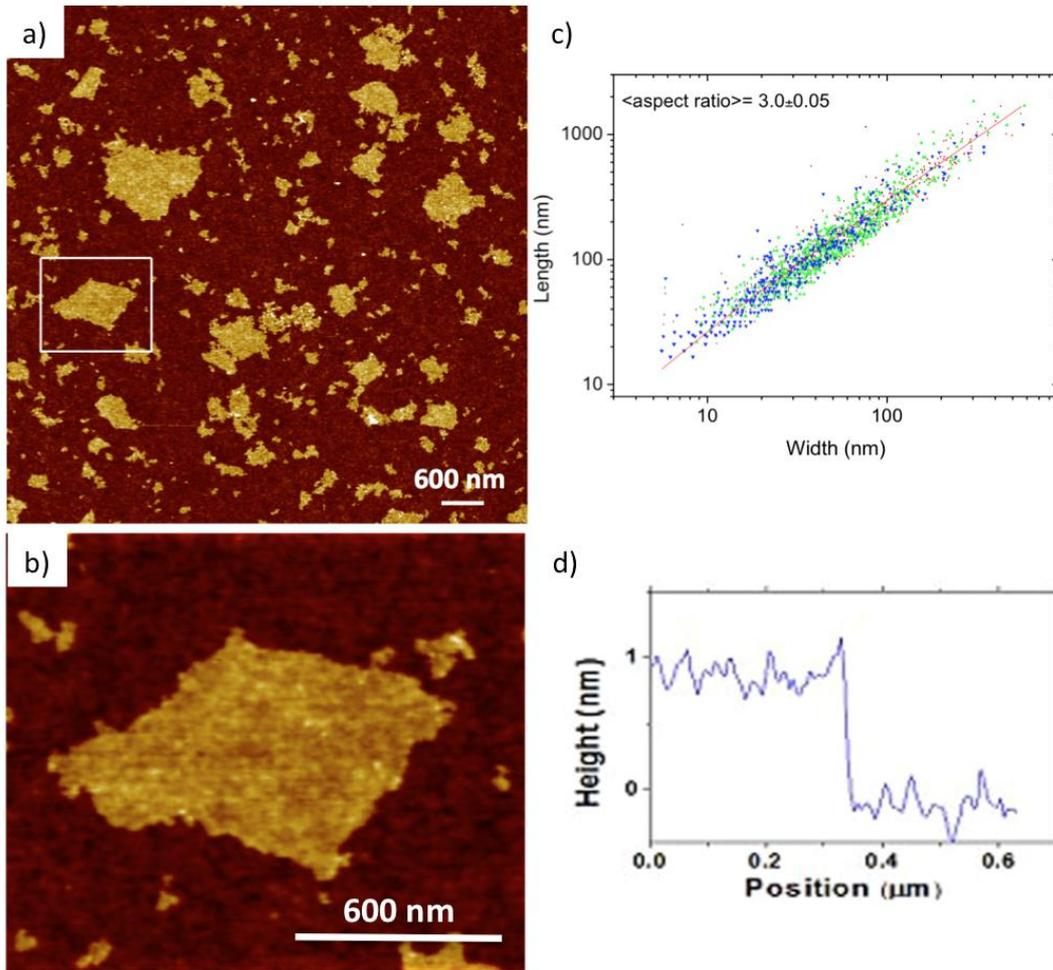
**Figure 2.** a,b) AFM image of GO sheets spin coated on silicon. c) Statistical analysis of the length/width ratio of the GO sheets, in log-log scale. The different colors of the points in the plot correspond to four different samples that were analyzed. d) Height profile taken along the dashed line in b).
