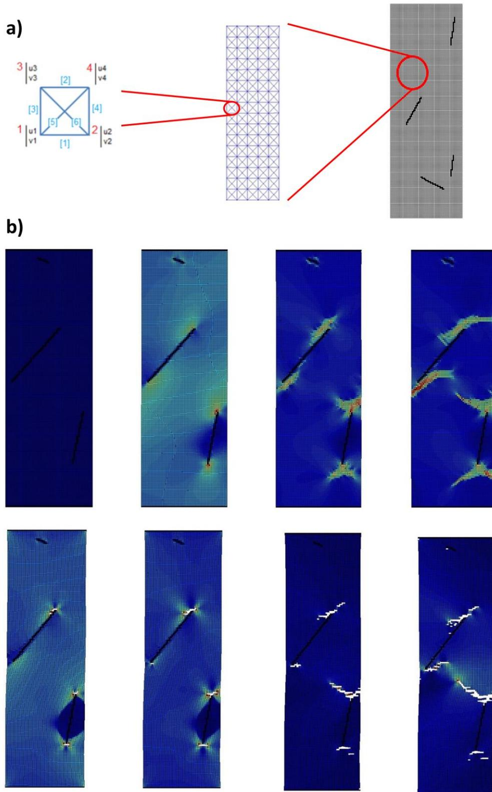
**Figure 10:** a) Schematic of the quadrilateral elements used in the model and FEM mesh of a typical GO-gelatin nanofibre specimen. Nodal degrees of freedom ( $u_i, v_i$ ) are also indicated; b) Development of crack propagation leading to nanofibre failure at the
