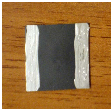
Figure S1 2x2 cm 2 sample for electrical conductivity measurements.
