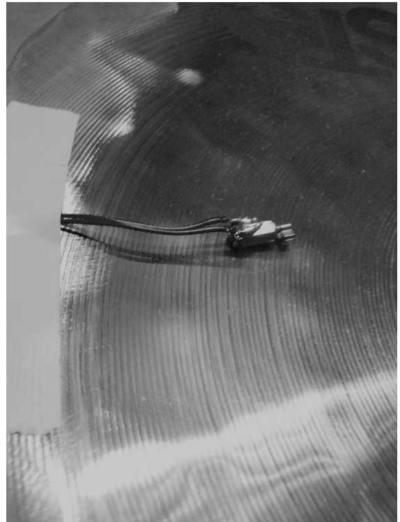
Figure 1. Minimal example: a cymbal and the vibrating mechanism from a mobile phone.
