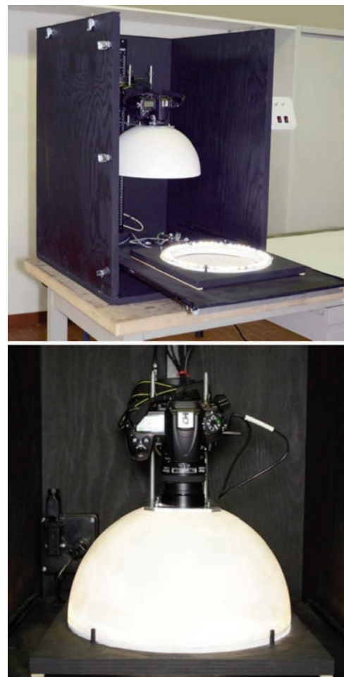
Figure 1. The Computer Vision System (without front and top walls) in which camera and the white hemisphere are lifted up to allow samples arrangement (on left); the same system during image acquisition (on right).
