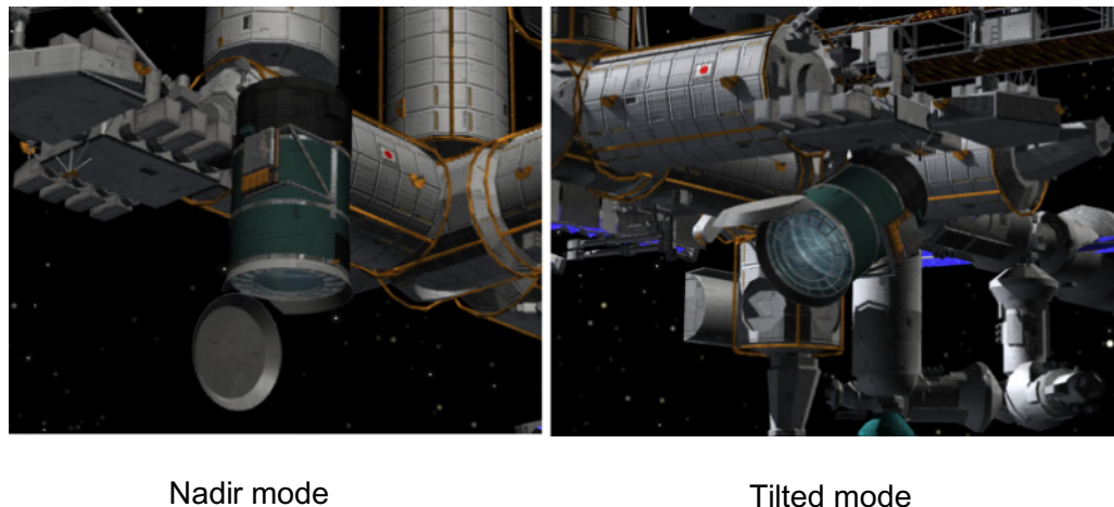
Figure 2. Artist's illustration of the JEM-EUSO telescope attached to the JEM of the ISS.
