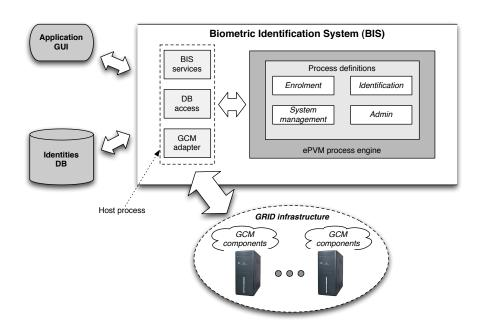
Figure 4 BIS high-level architecture
