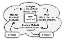
Figure 2 The classical control loop implemented within Autonomic Managers in GCM Behavioural Skeletons
