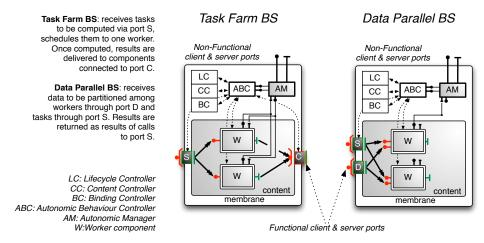
Figure 3 Behavioural skeletons currently implemented in GCM
