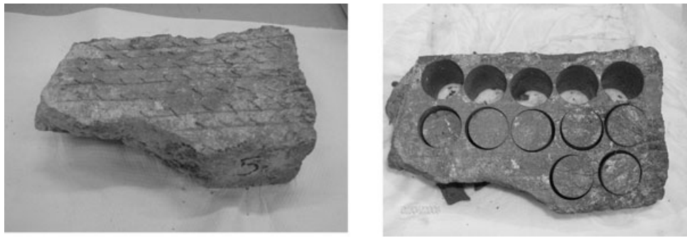
Figure 1. Brick sample from Saluzzo. Samples were drilled perpendicular to their flat surface.
