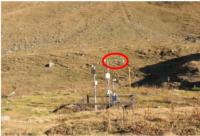
Fig. 4 Automatic nivo-meteorological station, the red circle denotes the snow sensor
