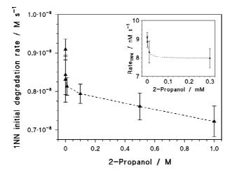
**Figure 5.** Initial transformation rates of 0.1 mM 1NN as a function of the concentration of 2-propanol. UVA irradiation, pH 6.5, aerated solution. <sup>25</sup> The insert shows the rate trend for 2-propanol concentration values up to 0.3 mM. The dashed curve is the fit of the experimental data with  $Rate_{INN} = R_{INN,\bullet OH}(equation 7) + c$ .
