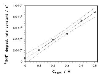
**Figure 3.** Pseudo-first order degradation rate constant of  ${}^{3}1NN^{*}$ , 60 produced upon irradiation of 0.1 mM 1NN, as a function of the concentration of added NaOH. Laser pulse: 60 mJ, 355 nm, aerated solution. Error bars derived at the  $3\sigma$  level simply from the scattering of the experimental data. Regression line is dashed, 95% confidence bands are dotted.
