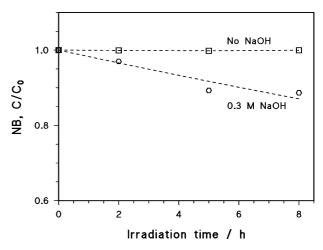
Figure 7. Time evolution of 0.01 mM NB upon UVA irradiation of 0.1  $^{65}$  mM 1NN + 0.3 M NaOH, and of 0.1 mM  $H_2O_2$  + 0.3 M NaOH. Irradiation was carried out in aerated solution.
