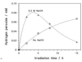
Figure 6. Time trend of  $H_2O_2$  upon UVA irradiation of 0.1 mM 1NN and 0.01 mM NB in aerated solution, without NaOH and with 0.3 M NaOH.
