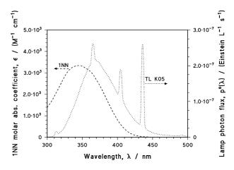
**Figure 1.** Spectral photon flux density  $p^{\circ}(\lambda)$  of the adopted UVA lamp. Molar absorption coefficient  $\varepsilon$  of 1NN.
