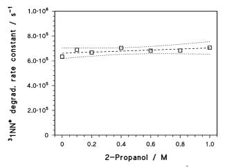
**Figure 4.** Pseudo-first order degradation rate constant of <sup>3</sup>1NN\* as a function of the concentration of 2-propanol. Laser pulse: 60 mJ, 355 nm, pH 6.5, aerated solution. Error bars derived at the  $3\sigma$  level simply from 15 the scattering of the experimental data. Regression line is dashed, 95% confidence bands are dotted.
