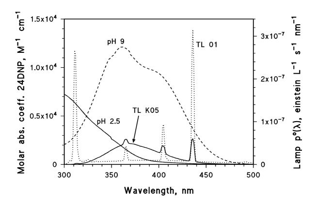
**Figure 1.** Absorption spectra (molar absorption coefficients) of 24DNP at pH 2.5 and 9 (adjusted with HClO<sub>4</sub> and NaOH, respectively). Emission spectra (spectral photon flux densities) of the lamps adopted for the irradiation experiments, TL01 (dotted trace) and TL K05 (solid trace).
