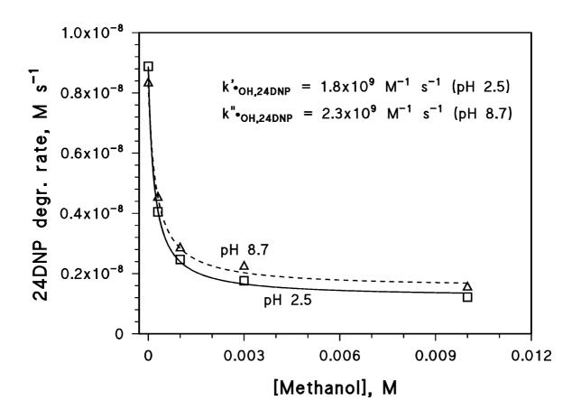
**Figure 3.** Initial degradation rates of 0.1 mM 24DNP upon irradiation of 0.1 M NaNO<sub>3</sub> under the TL 01 lamp (UVB), as a function of the concentration of methanol.
