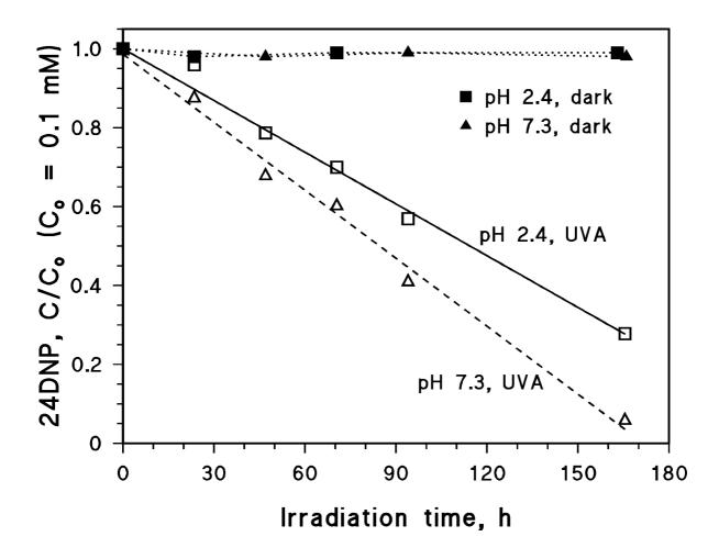
Figure 2. Time evolution of 0.1 mM 24DNP, upon irradiation under the TL K05 lamps (UVA) and in the dark. The pH values of 2.4 and 7.3 were adjusted upon addition of  $HClO_4$  and NaOH, respectively.
