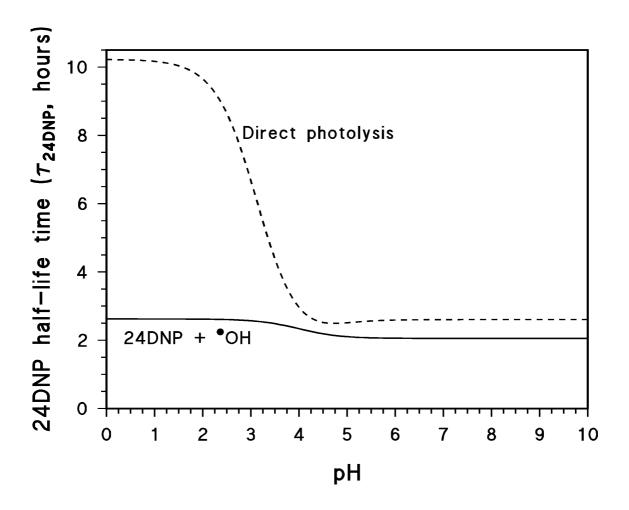
**Figure 4.** Half-life times of 24DNP as a function of pH, because of direct photolysis and the reaction with <sup>•</sup>OH. It was adopted [ $^{\bullet}OH$ ] =  $3.8 \times 10^{-14}$  M, relevant to the atmospheric aqueous phase under a sunlight UV irradiance of 22 W m<sup>-2</sup>.
