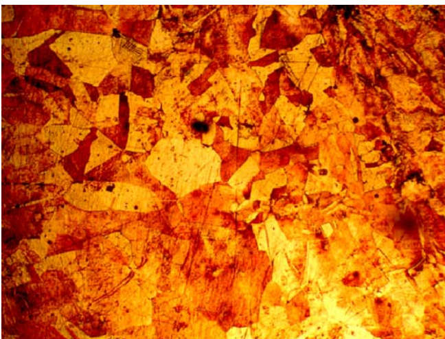
FIGURE 5 Photomicrograph (x80) of the body of the Savignano 994 sample showing a regular grain distribution characterized by twin lines typical of recrystallisation
