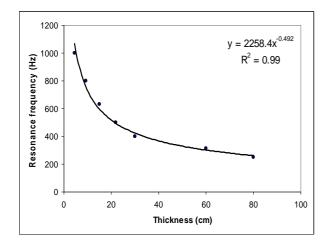
Figure 11: Cavity thickness vs. resonance frequency of the absorption peaks
