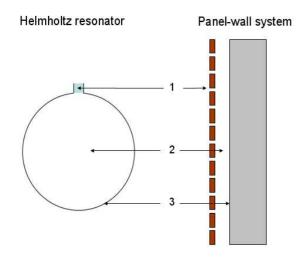
**Figure 4:** Longitudinal section of a Helmholtz resonator (left) and a system made of perforated panel and wall (right). 1 is the neck in the resonator, corresponding to the holes in the wood-based panel; 2 is the cavity, corresponding to the empty space between panel and wall; 3 is the cavity surface, which corresponds to the wall
