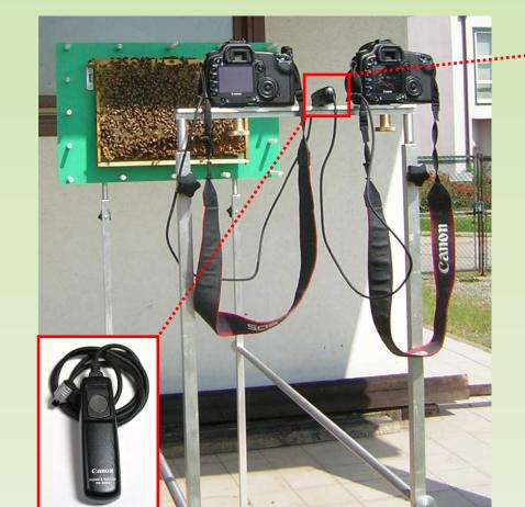
If the subject is a moving one (like honey bees) the stereopair must be acquired simultaneously by means of synchronizing device and remote controller.
