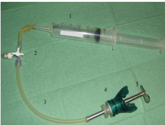
Figure 1. Illustration of oral NO device. Syringe with NO-free air (1); two-way valve for delivery and withdrawal of air sample to and from the oral cavity and to the NO meter (2); wide-bore teflon tube (3); soft mouthpiece (4); Holed metal tube welded at a right angle to a shaped plate (5).
