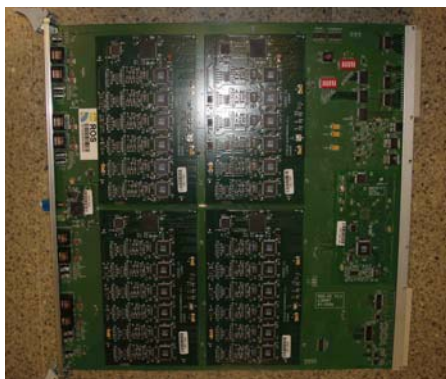
Figure 4: Read-Out Server (ROS) board.
