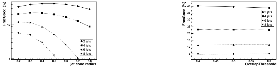
Fig. 46: Fraction of well clustered and selected events versus Fig. 47: Fraction of well clustered and selected events versus the cone radius for a merging threshold of 0.5 and a cone area the threshold for merging for a cone radius of 0.3 and an area fraction of 0.25 (MC algorithm).
