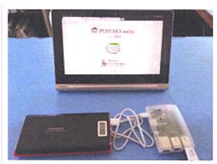
Figure 2: Current prototype of the Library-in-a-Box system
