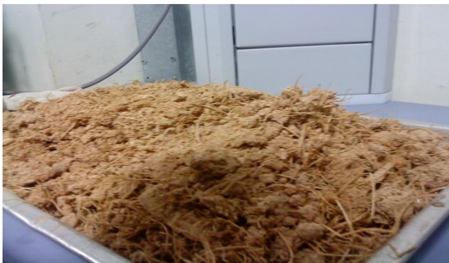
Figure 2: The sago hampas used for adsorption of humic substances
