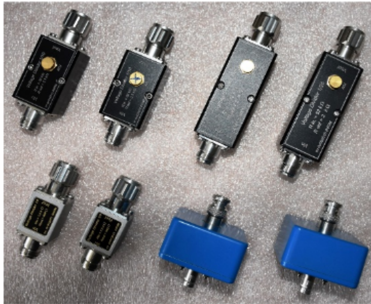
Figure 1.36: Set of wideband coaxial compensated RVD for voltage scaling with ratio from 1:3 to 1:52 constructed at INRIM.
