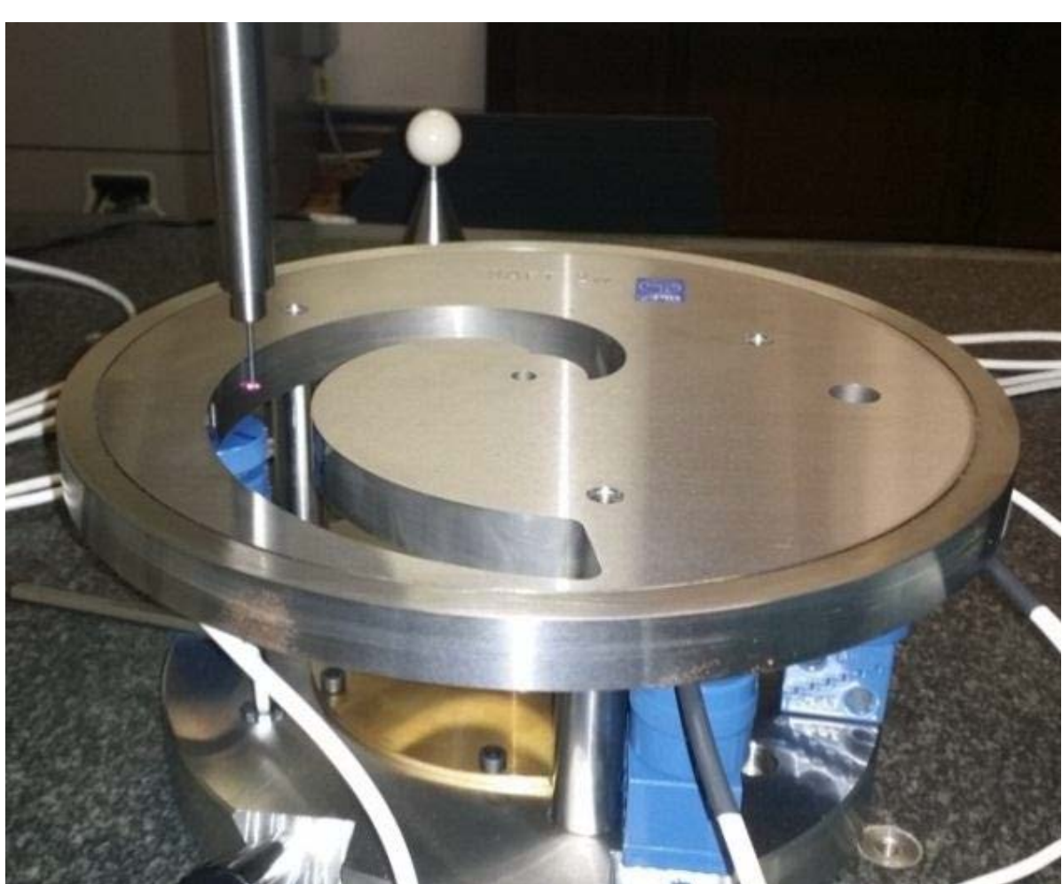
Example of internal involute measurement scanning
