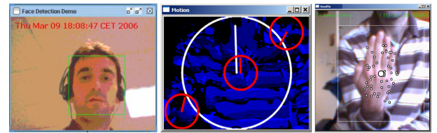
Figure 4: Screenshots of three visual input modality components: face detector, motion detector, and gesture recogniser.
