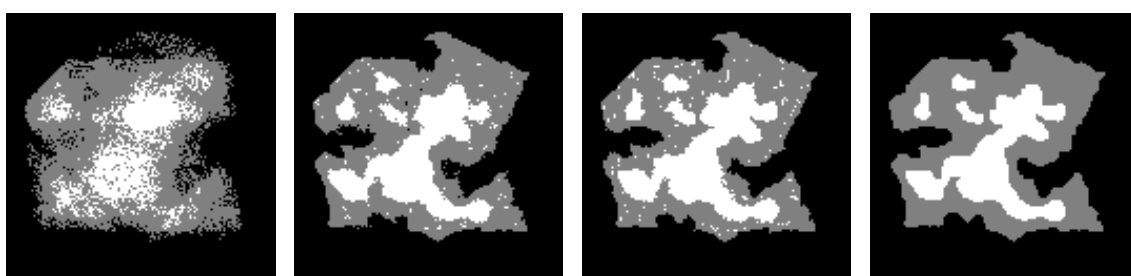
(d) Phantom 5(c). Alg. 1 with \tau = \frac{1}{\sqrt{128}} . N. of projection angles: left: 4; middle-left: 16; middle-right: 20; right: 24.
