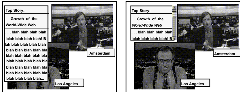
(a) unconstrained growth of an HTML text object (b) constrained growth of an HTML text object
