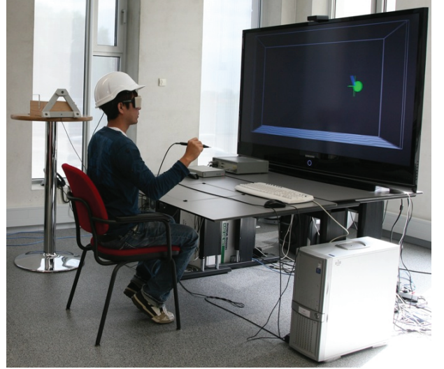
Figure 1: The experimental environment: a head tracked stereo display and a 6DOF input stylus. Several depth cues were created during the experiment, including the stereoscopic viewing, head tracking, head lighting, wire-frame box and the chessboard pattern floor.
