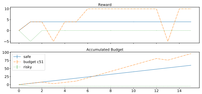
Figure 4: Top: the rewards received by an agent following an optimistic budget-aware policy for 15 episodes, as estimated by Eq. 5. Bottom: the corresponding accumulated budget. The risky agent runs out of budget immediately, while the budget-aware agent modifies its policy according to its resources.
