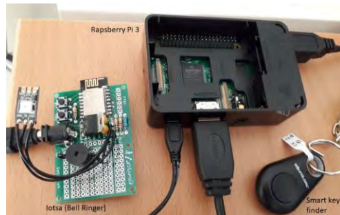
Figure 14 – Raspberry Pi 3, Iotsa (bell ringer) and smart key finder used to implement the Igor access control framework design
