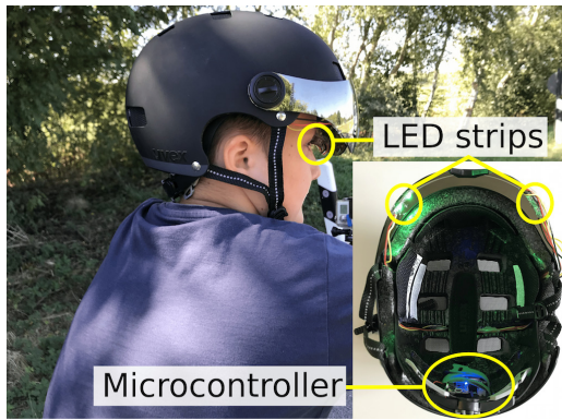
Figure 8: LED helmet with LED strips integrated into the visor for the light navigation in the test-track study.
