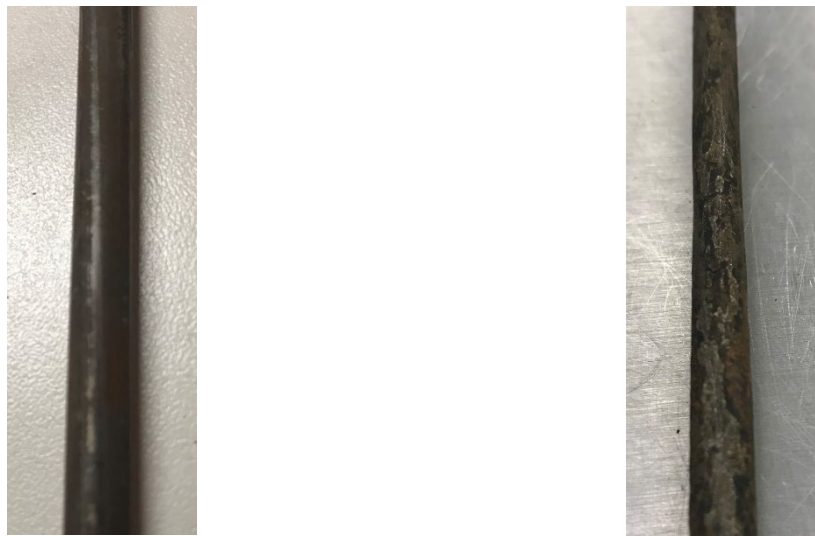
Figure 3.3: Reinforcing bars before (left) and after (right) the HCL treatment
