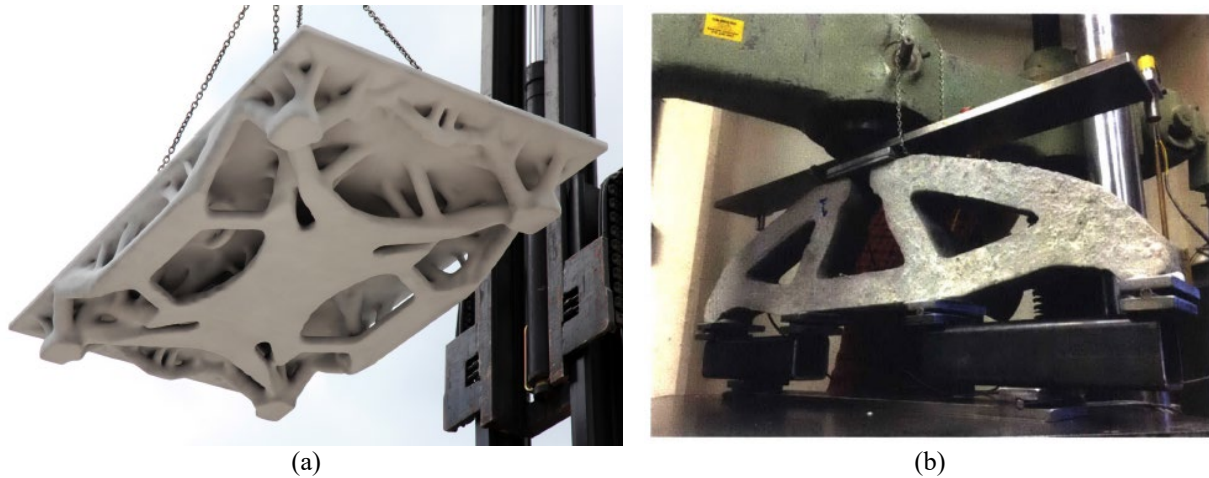
Figure 2.2: Topology optimized (a) UHPFRC slab with four supports (Jipa et al., 2016) and (b) PC beam testing under compression (Jewett and Carstensen, 2019)
