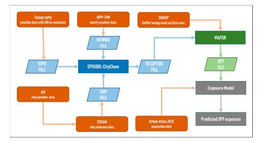
**Figure 1.** Outline of the sequential processing chain developed in this study. The brown and blue colors refer to the various input datasets and their initial processing, and the atmospheric dispersion and transformation modeling, respectively. The modeling of the aerosol processes and the exposure modeling together with the final product are presented with green and grey colors.
