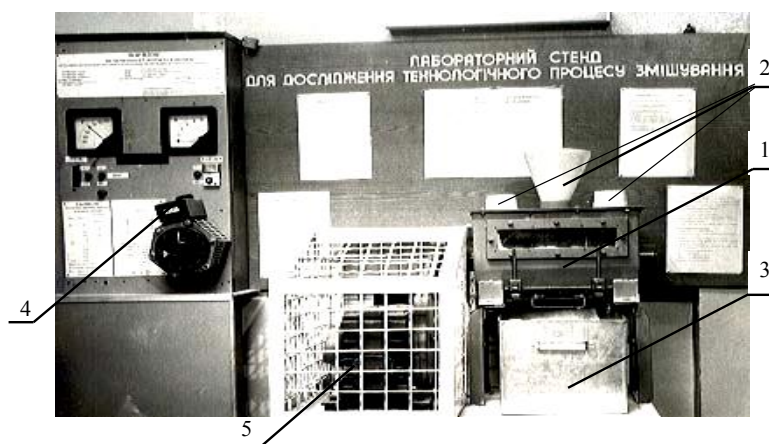
Fig. 3. Laboratory stand for study of technological mixing process: 1 – mixer, 2 – loading pipes, 3 – unloading tray, 4 – control desk, 5 – electricity cable
