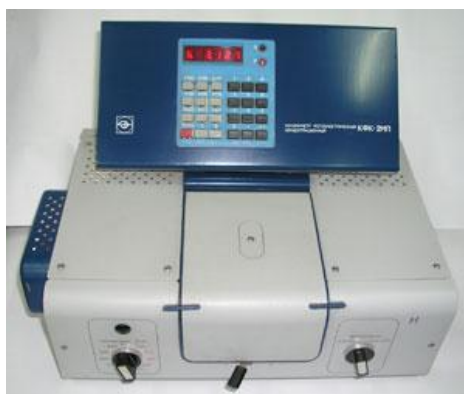
Fig. 15. Photoelectrocolorimeter KPC-2MP (“ZOMF”, Russia)
